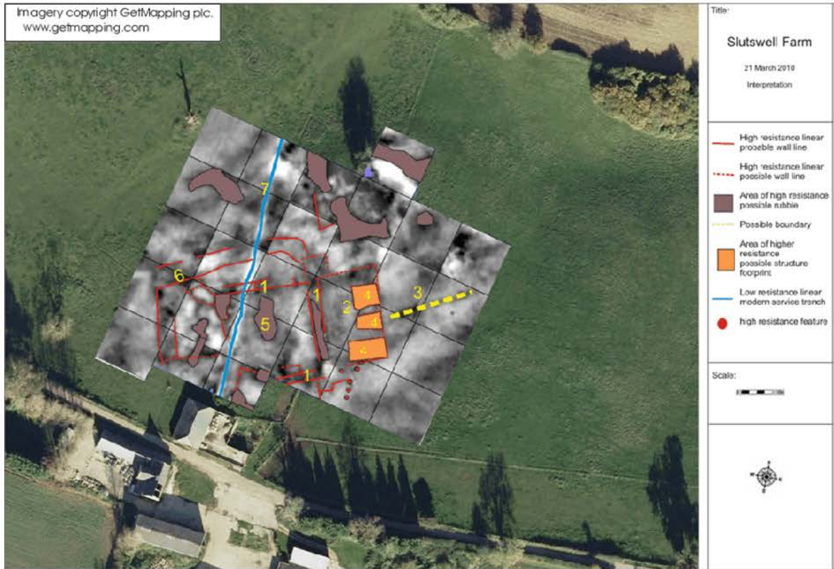
Figure 6 Interpretation of resistance results (geophysics results © A. J. Roberts superimposed on air photo)
